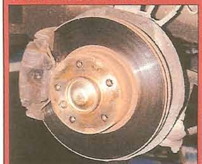
Sometimes you could be burning fuel needlessly because you're inadvertently slowing the car down due to binding brakes. So it's always worth checking these on a regular basis.
