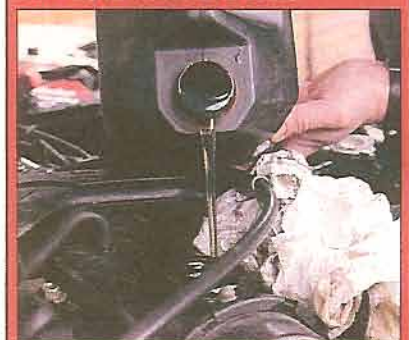
As a general rule, older, less advanced engines require a thicker grade motor oil, whereas modern multi-valve engine require lighter, semi-synthetic or fully synthetic lubricant.
