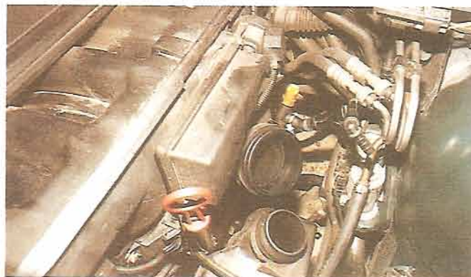
With the intake pipework out of the way, the vacuum piping is visible.
