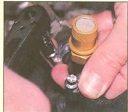
Fit the device in between the two sections of pipe and seal up by tightening two jubilee clips (these are not provided).
