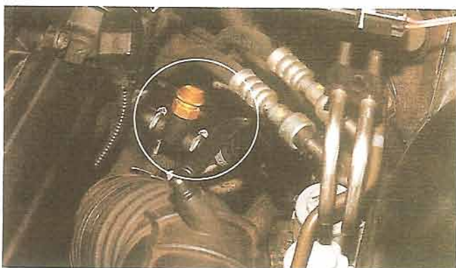
The Ecotek is installed between the manifold and the brake servo non-return valve.
