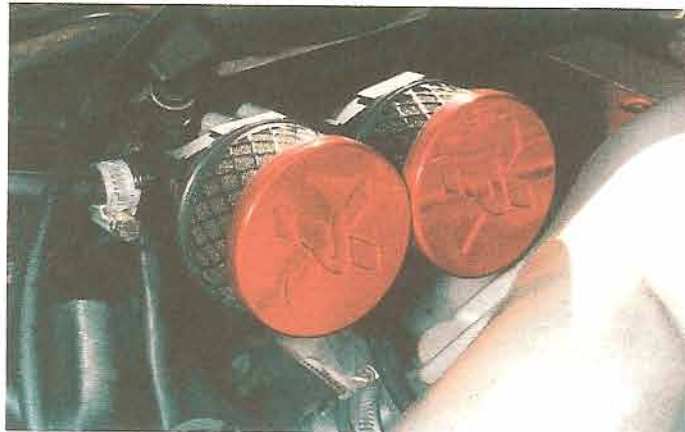
The finished job, with the Pipercross filter/silencer units added. Now for the driving test...
