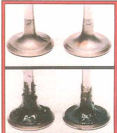
Particularly important on modern multi-valve engines is the choice of motor oil. If you opt for the wrong one, the result could be valve stick.
