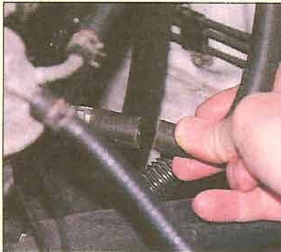
Locate the vacuum servo pipe that runs between the brake servo and the inlet manifold. Cut through the pipe with a sharp blade.
