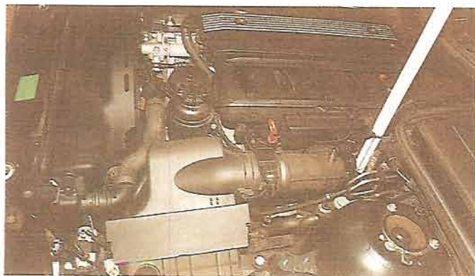
The E39 engine bay isn't for the faint-hearted but access to the servo is pretty easy.
