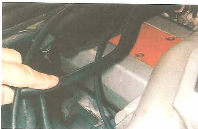
On this Vauxhall Senator, proper fitting involved cutting this tube and reconnecting it carefully afterwards
